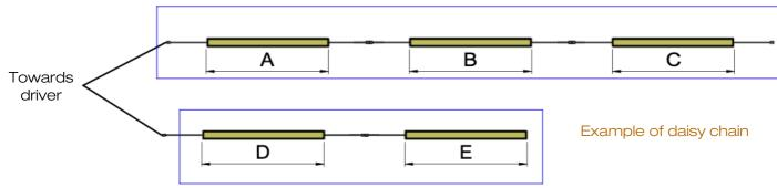
Create as many lines as needed to respect the maximum length per line, according to the selected LED strip and the wattage of the driver
