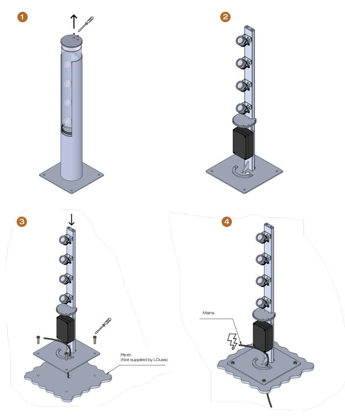
All the connections have to be made before powering up, otherwise the luminaires could be seriously damaged.
