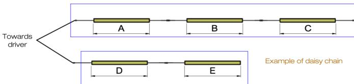
Create as many lines as needed to respect the maximum length per line, according to the selected LED strip and the wattage of the driver
