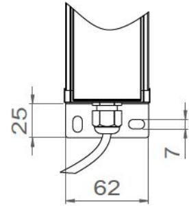
Adjustable spacing fixing brackets
