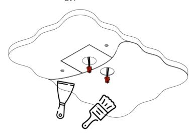
**3.** Cover the gypsum board and brackets with plaster and painting
