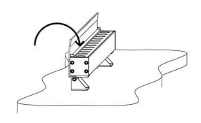
All the connections have to be made before powering up, otherwise the luminaires could be seriously damaged.
