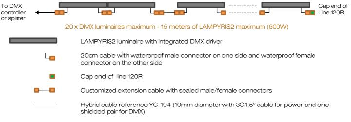
Maximum total cable length from DMX controller (or splitter) to last luminaire = 300m Beyond that, a repeater or splitter is required
